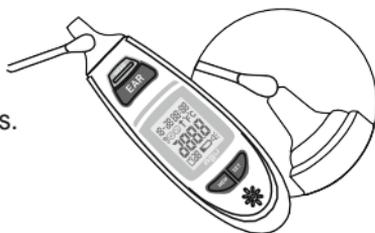
**Lens/measuring sensor:** In case of contamination of the infrared thermometer sensor lens, the readings begin to change immediately as something interferes with the measurement (usually the readings are too low). To eliminate this problem, it is enough to wipe the sensor with a soft lint-free cloth (or cotton swab) moistened with disinfectant solution. Then it is necessary to wipe the lens with a dry soft lint-free cloth. After the cleaning procedure, the lens surface should be
